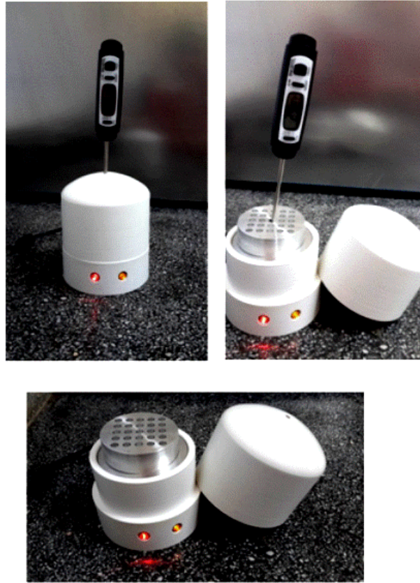
Plate 7. Fabricated heat block called “Lab in a Mug”
